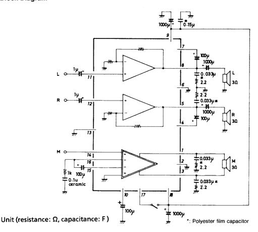
Note 1 : The motor should not be connected to the power switch pin, since transient noise may appear on the amplifier outputs when the motor is started or stopped.
