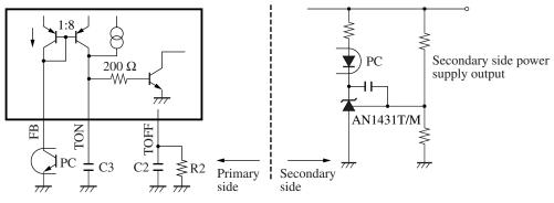
Figure 3. Power supply output control system
