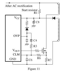
terminal is outputted. By this voltage, the charge current flows into the C4 and the CLM terminal voltage rises. The CLM terminal voltage decreases with the lapse of time since it changes in proportion to the charge current of the C4. The CLM circuit operates by the sum of the voltage across the both ends of R7 created by the current flowing into the power MOSFET when turning on power and the voltage across the both ends of R6 created by the charge current of the C4.
