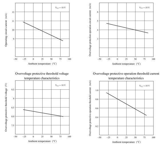
Overvoltage protective threshold voltage temperature characteristics
