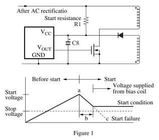
Since the supply voltage continuously decreases during the above period (area b in figure 1), the power supply is not able to start (state c in figure 1), if the stop voltage of the IC is reached before the sufficient supply voltage is supplied from the bias coil.
