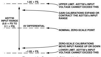
Figure 16. Span and Offset Limits
