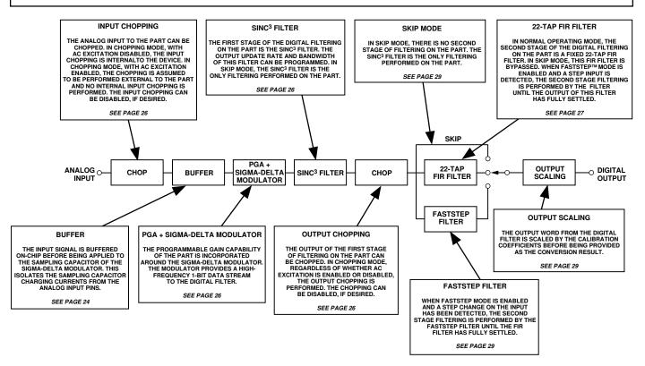
Figure 3. Signal Processing Chain
