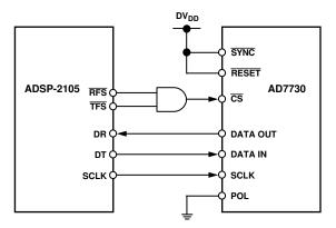
Figure 22. AD7730 to ADSP-2105 Interface
