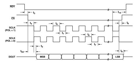
Figure 18. Read Cycle Timing Diagram
