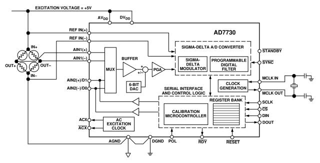
Figure 23. Typical Connections for DC-Excited Bridge Application
