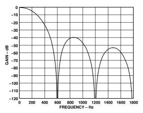
Figure 10. Frequency Response of First Stage Filter
