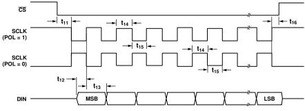
Figure 19. Write Cycle Timing Diagram
