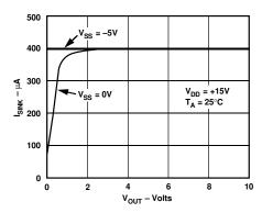
Figure 2. Variation of  $I_{SINK}$  with  $V_{OUT}$
