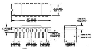
NOTES: 1. LEAD NO. 1 IDENTIFIED BY DOT OR NOTCH. 2. CERAMIC DIP LEADS WILL BE EITHER GOLD OR TIN PLATED IN ACCORDANCE WITH MIL-M-38510 REQUIREMENTS.
