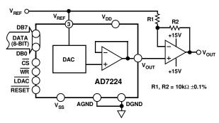
Figure 6. Bipolar Output Circuit
