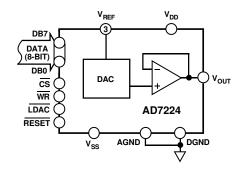
Figure 5. Unipolar Output Circuit
