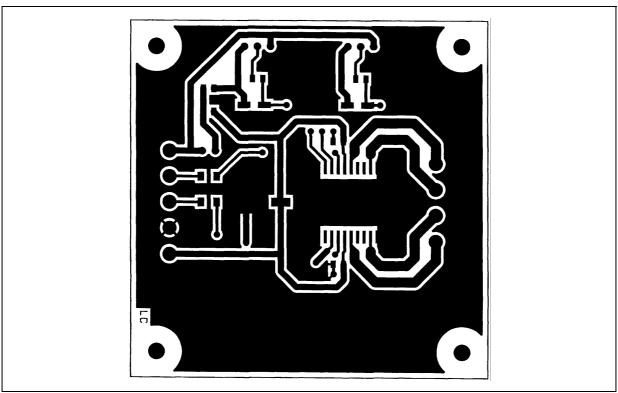
Figure 16. Evaluation Board Bottom Layer Layout
