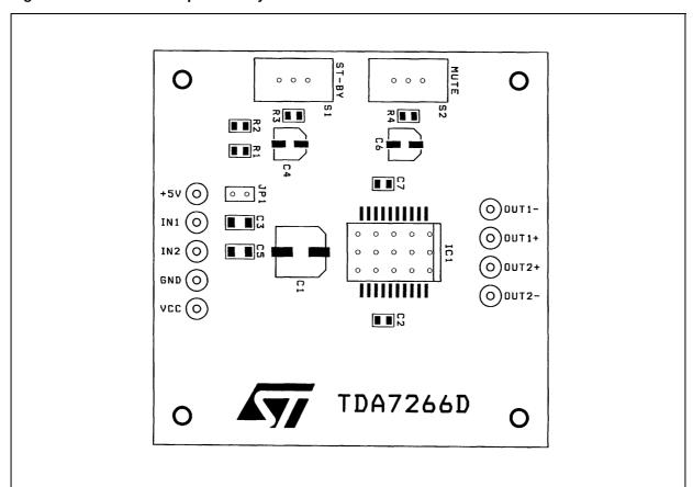
Figure 15. Evaluation Board Top Layer Layout
