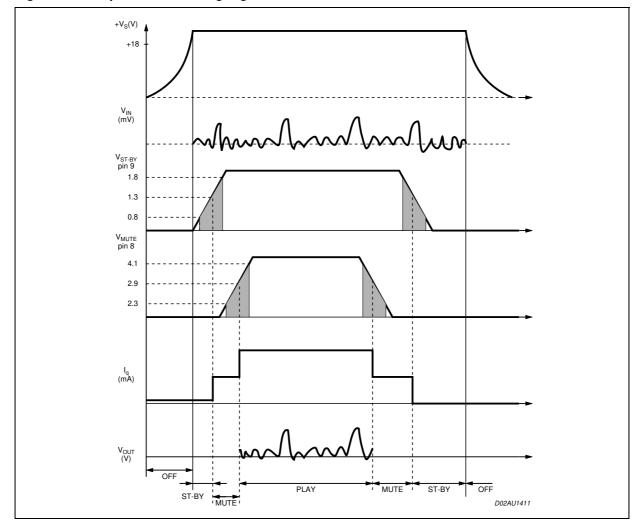
Figure 2. Microprocessor Driving Signals
