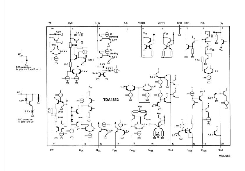
Fig.9 Internal circuits.
