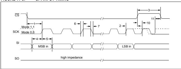
FIGURE 11-9: SPI OUTPUT TIMING
