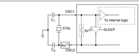
Note 1: A series resistor, Rs, may be required for AT strip cut crystals.
