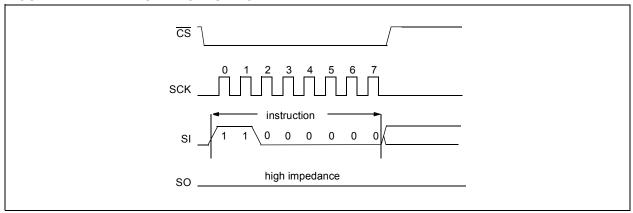
FIGURE 11-8: SPI INPUT TIMING
