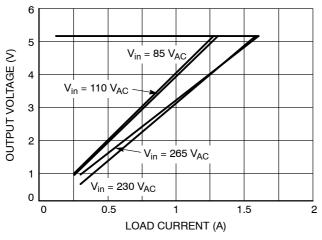
Figure 32. Converter Load Regulation
