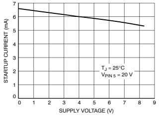
Figure 21. Startup Current versus Supply Voltage
