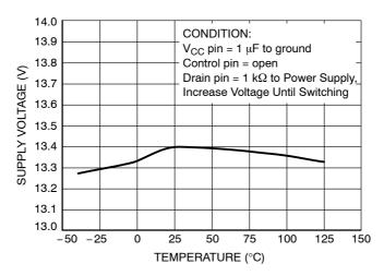
Figure 27. Supply Voltage versus Temperature
