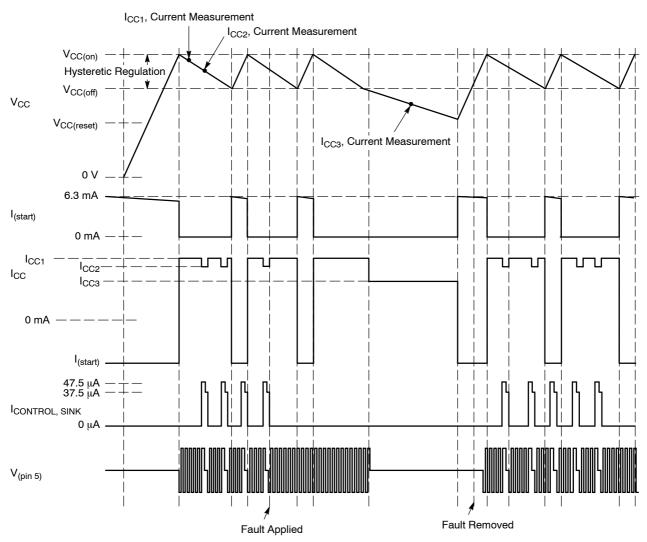
Figure 4. Non-Latching Fault Condition Timing Diagram
