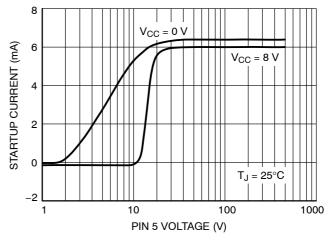
Figure 22. Startup Current versus Pin 5 Voltage
