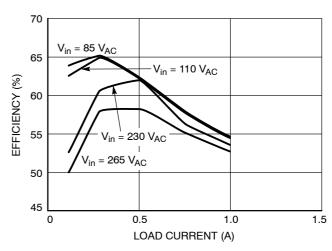
Figure 37. Charger Efficiency
