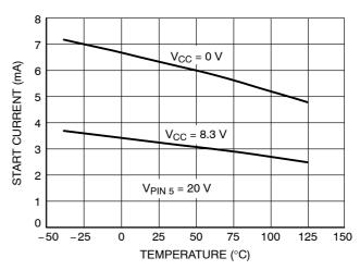
Figure 20. Start Current versus Temperature
