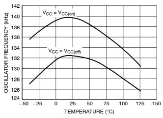
Figure 7. Oscillator Frequency (136 kHz Version) versus Temperature
