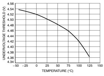
Figure 19. Undervoltage Lockout Threshold versus Temperature
