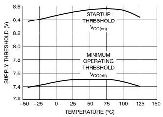
Figure 18. Supply Voltage Thresholds versus Temperature
