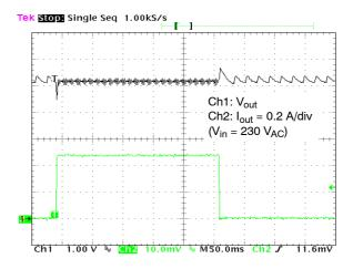
Figure 35. Charger Load Transient Response
