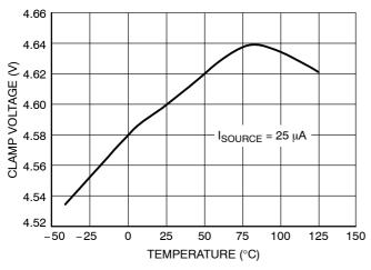
Figure 13. Control Input Upper Window Clamp
