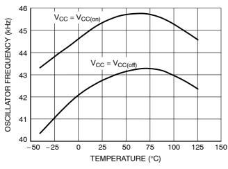
Figure 5. Oscillator Frequency (44 kHz Version) versus Temperature
