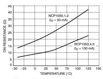
Figure 14. On Resistance versus Temperature
