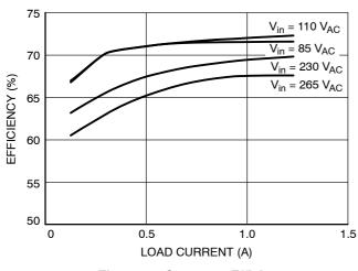
Figure 36. Converter Efficiency
