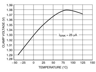
Figure 12. Control Input Lower Window Clamp
