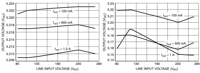
Figure 30. Converter Line Regulation
