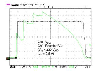
Figure 38. Converter On/Off Line Transient Response
