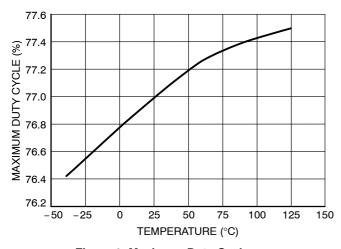
Figure 9. Maximum Duty Cycle versus Temperature
