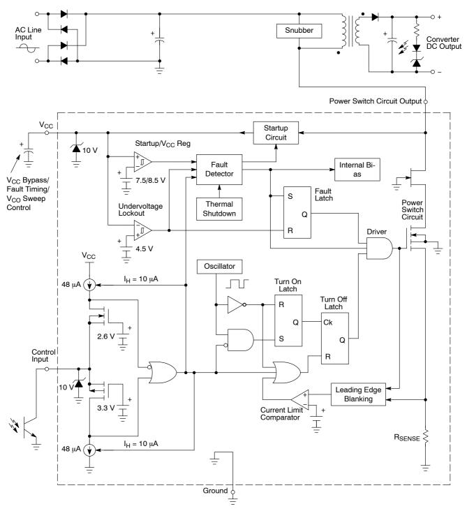
Figure 2. Representative Block Diagram
