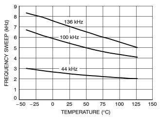
Figure 8. Frequency Sweep versus Temperature
