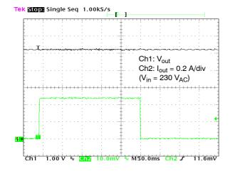
Figure 34. Converter Load Transient Response
