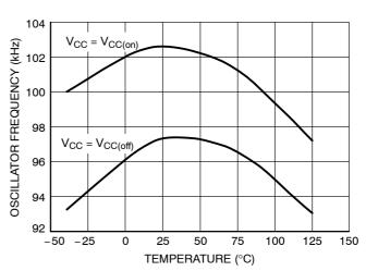
Figure 6. Oscillator Frequency (100 kHz Version) versus Temperature
