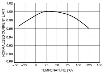
Figure 17. Normalized Peak Current Limit versus Temperature
