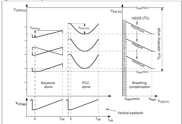
Figure 13. EWOut output waveforms
