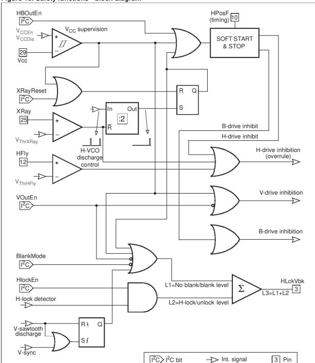
Figure 15. Safety functions - block diagram
