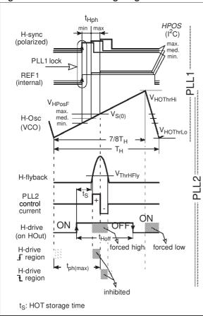
Figure 8. HFly input configuration
