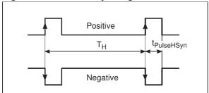
Figure 3. Extraction of V-sync signal from H/V-sync signal
