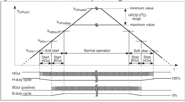
Figure 10. Control of HOut and BOut at start/stop at nominal V<sub>cc</sub>
