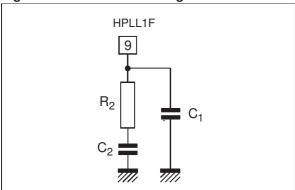
The PLL1 is internally inhibited during extracted vertical sync. pulse (if any) to avoid taking into account missing or wrong pulses on the phase comparator. Inhibition is obtained by forcing the charge
