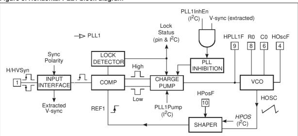
Figure 6. Horizontal oscillator (VCO) schematic diagram
