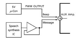
(Fig.7) The application of AUX. amplifier
