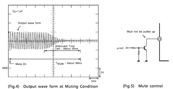
The attenuation by the muting function is 70 dB (typ.). This muting is very smooth attenuating by the time constant of pin(1): Smoothing.
