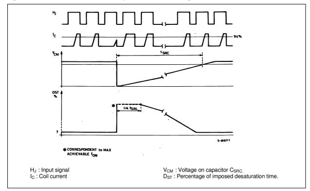
Figure 2: SRC: Icoil Failure and Time Dependence of Active Region.
