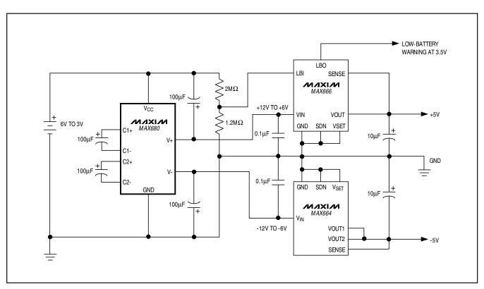
Figure 5. Regulated +5V and -5V from a Single Battery
