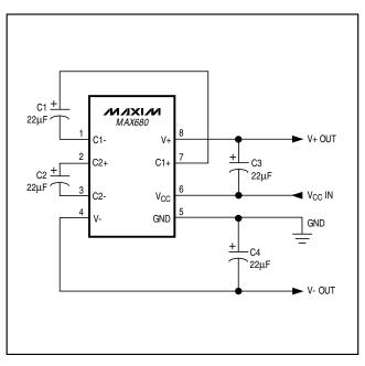
Figure 3. Positive and Negative Converter
