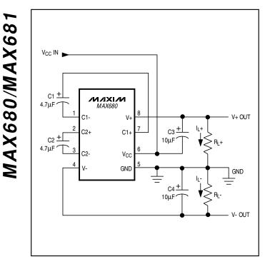
Figure 1. Test Circuit
