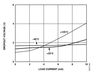
Figure 20. REF02 Dropout Voltage vs. Load Current
