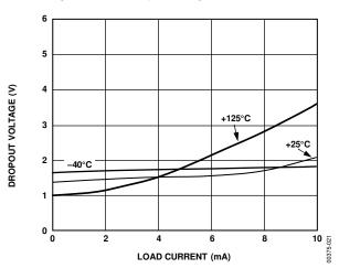
Figure 21. REF03 Dropout Voltage vs. Load Current
