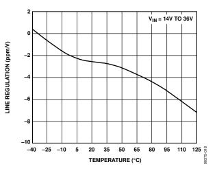
Figure 16. REF01 Line Regulation vs. Temperature
