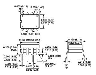
CONTROLLING DIMENSIONS ARE IN INCHES; MILLIMETER DIMENSIONS (IN PARENTHESES) ARE ROUNDED-OFF INCH EQUIVALENTS FOR REFERENCE ONLY AND ARE NOT APPROPRIATE FOR USE IN DESIGN.
