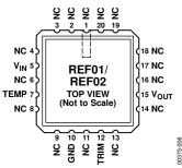
Figure 6. 20-Terminal LCC (RC-Suffix) Pin Configuration
