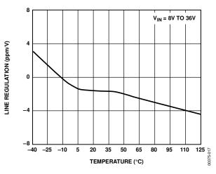
Figure 17. REF02 Line Regulation vs. Temperature
