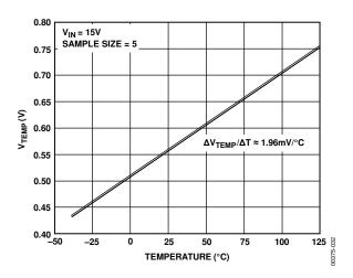
Figure 32. Output Voltage at TEMP Pin vs. Temperature
