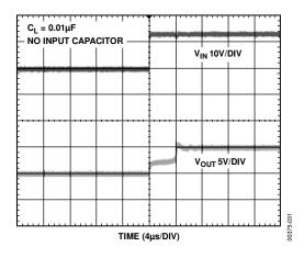
Figure 31. REF02 Turn-Off Response (No Input Capacitor)
