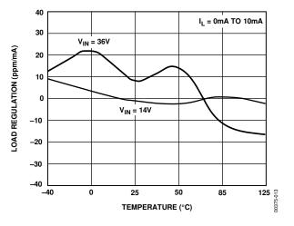
Figure 13. REF01 Load Regulation vs. Temperature
