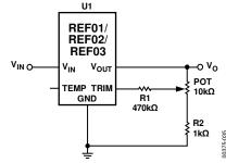
Figure 35. Optional Trim Adjustment Circuit
