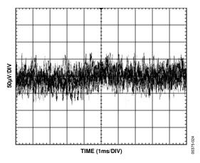
Figure 24. REF02 Typical Wideband Voltage Noise (10 Hz to 10 kHz)
