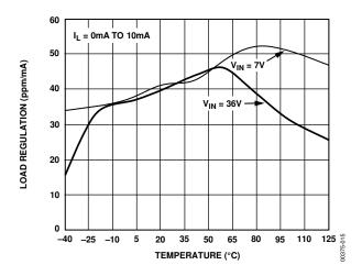
Figure 15. REF03 Load Regulation vs. Temperature
