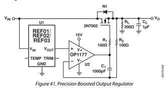
In this circuit, U2 forces V<sub>0</sub> to V<sub>REF</sub> by regulating the current through N1, thereby sourcing the load current directly from the input voltage source connected at V<sub>IN</sub>. Using the components shown, this circuit can source up to 50 mA with an input voltage of 15.0 V. The circuit's current sourcing capability can be further increased by replacing N1 with a higher-power MOSFET.
