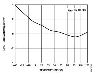
Figure 18. REF03 Line Regulation vs. Temperature
