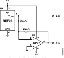
Figure 42. Bipolar Voltage Reference
