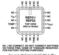
Figure 3. 20-Terminal LCC (RC-Suffix; 883 Parts Only)
