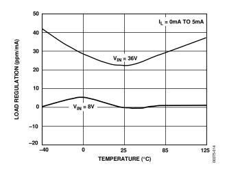
Figure 14. REF02 Load Regulation vs. Temperature
