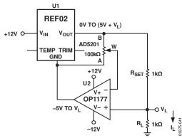
Figure 40. Programmable 0 mA to 5 mA Current Source
