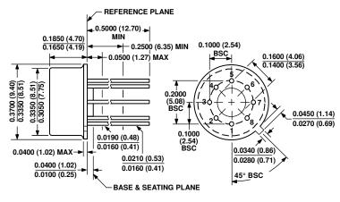
COMPLIANT TO JEDEC STANDARDS MO-002-AK CONTROLLING DIMENSIONS ARE IN INCHES; MILLIMETER DIMENSIONS (IN PARENTHESES) ARE ROUNDED-OFF INCH EQUIVALENTS FOR REFERENCE ONLY AND ARE NOT APPROPRIATE FOR USE IN DESIGN.
