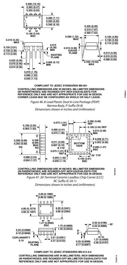
Figure 48. 8-Lead Standard Small Outline Package [SOIC\_N] Narrow Body, S-Suffix (R-8) Dimensions shown in millimeters and (inches)
