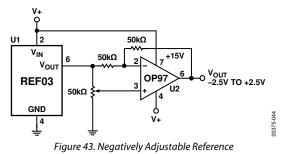
The voltage output from the op amp can be adjusted by changing the value of the potentiometer: as shown, the op amp outputs +2.5 V when the pot is pulled completely high, and -2.5V when pulled completely low. In this configuration, the load current is sourced by the op amp; therefore, a low offset op amp with a current rating that meets or exceeds the current requirements of the load should be used.
