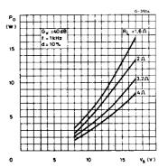
Figure 4. Output power vs. load resistance R<sub>L</sub>
