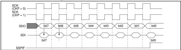
FIGURE 11-6: SPI MODE TIMING, SLAVE MODE WITH SS CONTROL
