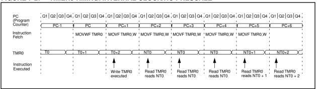
FIGURE 7-3: TIMER0 TIMING: INTERNAL CLOCK/PRESCALE 1:2
