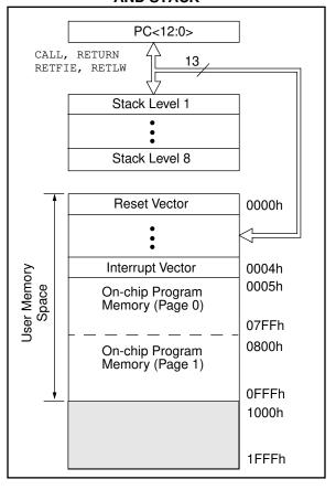
FIGURE 4-3: PIC16C76/77 PROGRAM MEMORY MAP AND STACK
