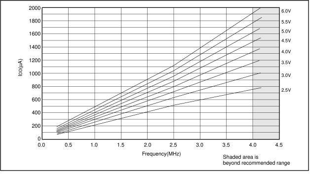
FIGURE 21-14: TYPICAL IDD vs. FREQUENCY (RC MODE @ 100 pF, 25°C)
