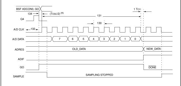
Note 1: If the A/D clock source is selected as RC, a time of Tcy is added before the A/D clock starts. This allows the SLEEP instruction to be executed.
