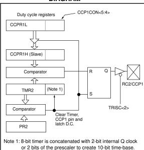
A PWM output (Figure 10-5) has a time base (period) and a time that the output stays high (duty cycle). The frequency of the PWM is the inverse of the period (1/period).
