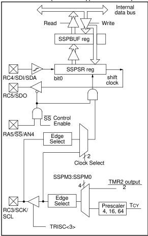
To enable the serial port, SSP Enable bit, SSPEN (SSPCON<5>) must be set. To reset or reconfigure SPI mode, clear bit SSPEN, re-initialize the SSPCON register, and then set bit SSPEN. This configures the SDI, SDO, SCK, and  $\overline{SS}$  pins as serial port pins. For the pins to behave as the serial port function, they must have their data direction bits (in the TRISC register) appropriately programmed. That is:
