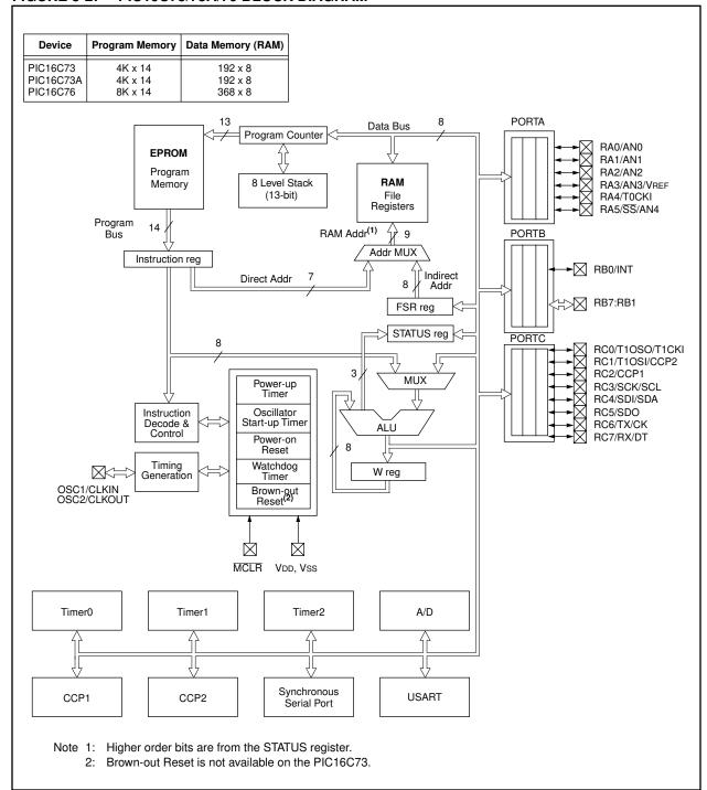
FIGURE 3-2: PIC16C73/73A/76 BLOCK DIAGRAM
