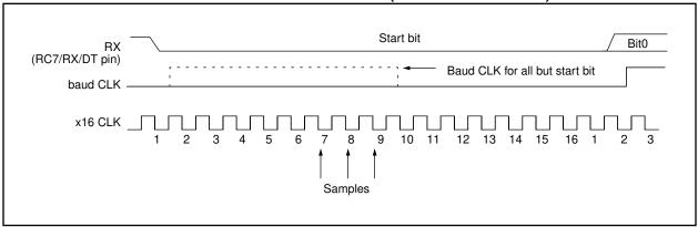
FIGURE 12-4: RX PIN SAMPLING SCHEME, BRGH = 1 (PIC16C73/73A/74/74A)
