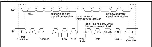
Figure 11-19 and Figure 11-20 show Master-transmitter and Master-receiver data transfer sequences.
