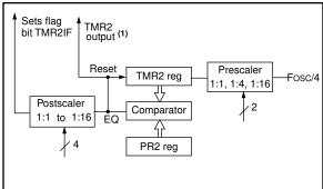
Note 1: TMR2 register output can be software selected by the SSP Module as a baud clock.
