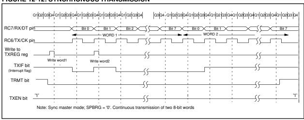
FIGURE 12-13: SYNCHRONOUS TRANSMISSION (THROUGH TXEN)
