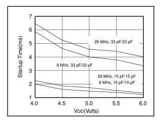
FIGURE 21-24: TYPICAL XTAL STARTUP TIME vs. VDD (XT MODE, 25°C)
