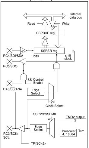
To enable the serial port, SSP enable bit SSPEN (SSPCON<5>) must be set. To reset or reconfigure SPI mode, clear enable bit SSPEN, re-initialize SSPCON register, and then set enable bit SSPEN. This configures the SDI, SDO, SCK, and  $\overline{SS}$  pins as serial port pins. For the pins to behave as the serial port function, they must have their data direction bits (in the TRIS register) appropriately programmed. That is:
