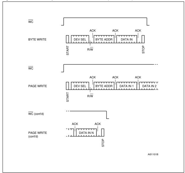
Figure 9. Write Modes Sequence with Write Control = 1 (ST24/25W02)
