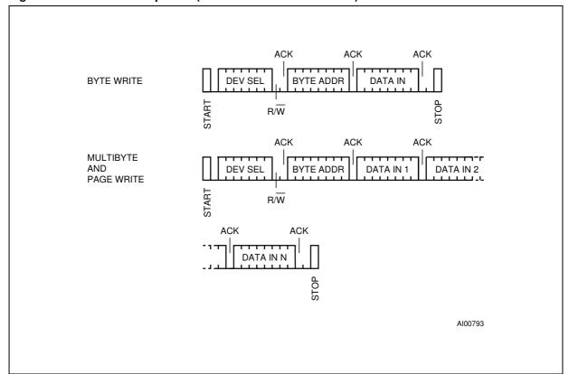
Figure 8. Write Modes Sequence (ST24/25C02 and ST24C02R)
