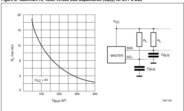
Figure 3. Maximum R<sub>L</sub> Value versus Bus Capacitance (C<sub>BUS</sub>) for an I<sup>2</sup>C Bus
