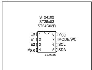
Figure 2B. SO Pin Connections
