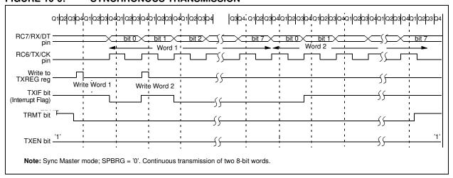
FIGURE 10-7: SYNCHRONOUS TRANSMISSION (THROUGH TXEN)
