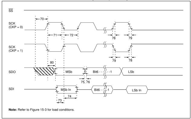
FIGURE 15-12: SPI MASTER MODE TIMING (CKE = 1, SMP = 1)
