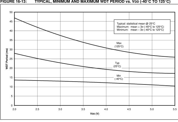
FIGURE 16-13: TYPICAL, MINIMUM AND MAXIMUM WDT PERIOD vs. VDD (-40°C TO 125°C)
