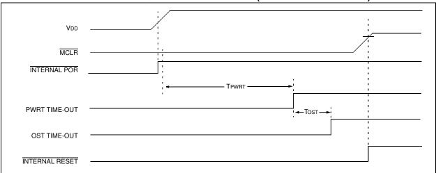
FIGURE 12-9: SLOW RISE TIME (MCLR TIED TO VDD THROUGH RC NETWORK)
