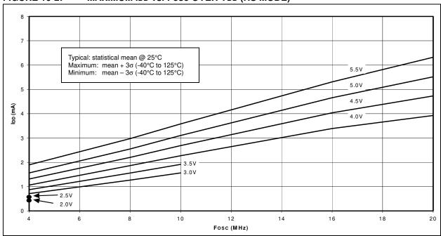
FIGURE 16-3: TYPICAL IDD vs. FOSC OVER VDD (XT MODE)
