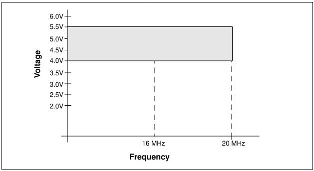
FIGURE 15-2: PIC16LF7X VOLTAGE-FREQUENCY GRAPH
