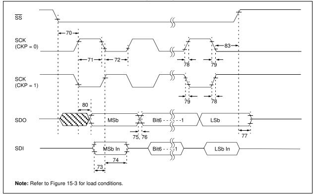
FIGURE 15-14: SPI SLAVE MODE TIMING (CKE = 1)
