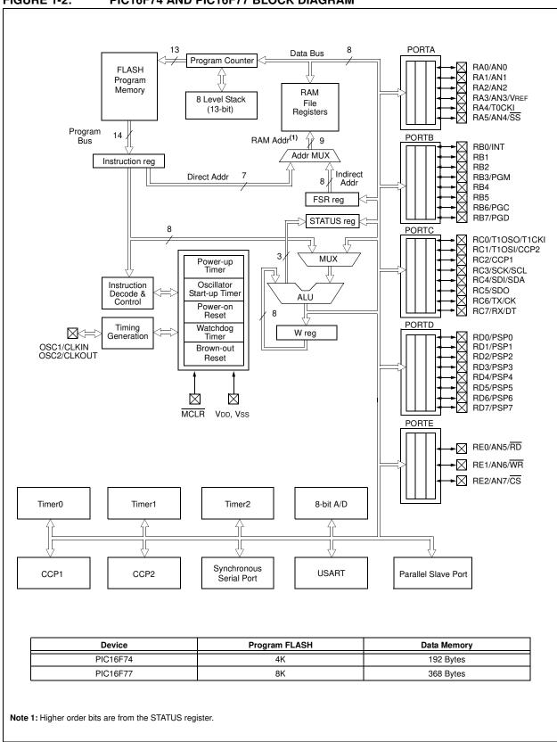
FIGURE 1-2: PIC16F74 AND PIC16F77 BLOCK DIAGRAM
