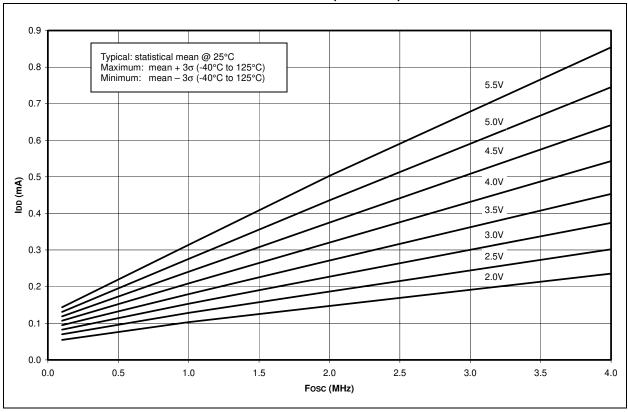
FIGURE 16-4: MAXIMUM IDD vs. Fosc OVER VDD (XT MODE)
