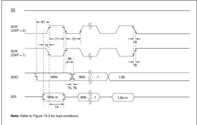
FIGURE 15-13: SPI SLAVE MODE TIMING (CKE = 0)
