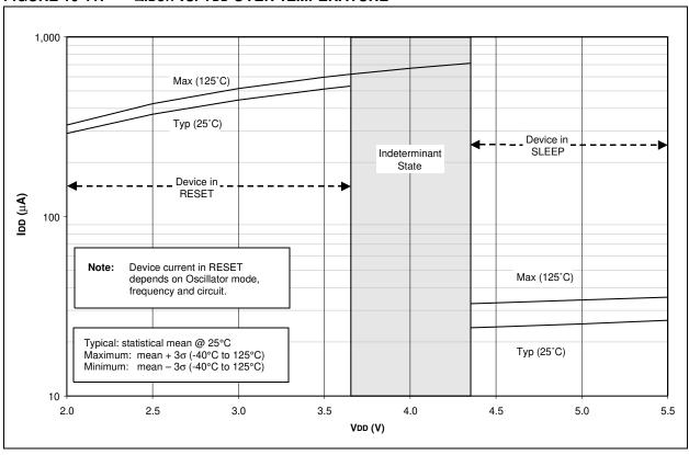
FIGURE 16-12: TYPICAL AND MAXIMUM AIWDT vs. VDD OVER TEMPERATURE
