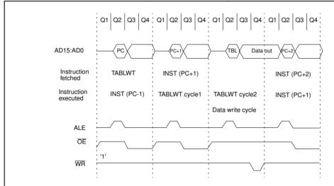
Note: If external write, and GLINTD = '1', and Enable bit = '1', then when '1' → Flag bit, Do table write.
