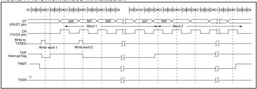
FIGURE 14-11: SYNCHRONOUS TRANSMISSION (THROUGH TXEN)
