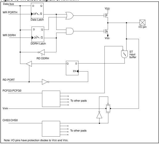
Figure 10-18:RH3:RH0 Block Diagram
