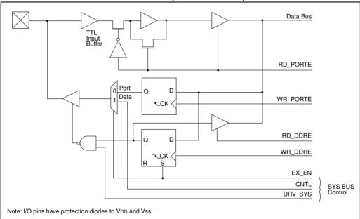
FIGURE 10-12: BLOCK DIAGRAM OF RE3/CAP4 PORT PIN
