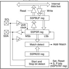
FIGURE 15-14: I<sup>2</sup>C MASTER MODE BLOCK DIAGRAM
