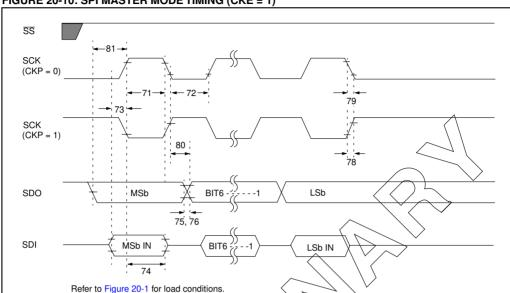
FIGURE 20-10: SPI MASTER MODE TIMING (CKE = 1)
