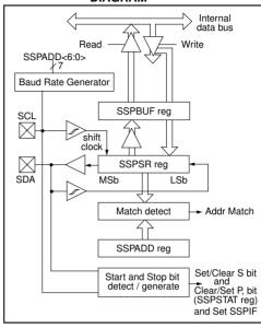
Two pins are used for data transfer. These are the SCL pin, which is the clock, and the SDA pin, which is the data. The SDA and SCL pins that are automatically configured when the I<sup>2</sup>C mode is enabled. The SSP module functions are enabled by setting SSP Enable bit SSPEN (SSPCON1<5>).
