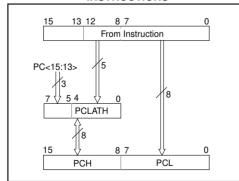
Using Figure 7-10, the operations of the PC and PCLATH for different instructions are as follows:
