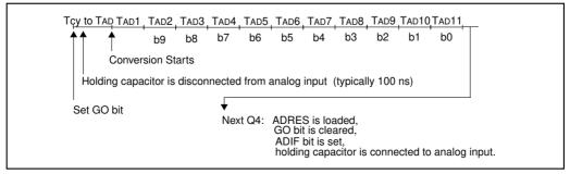
FIGURE 16-7: FLOWCHART OF A/D OPERATION
