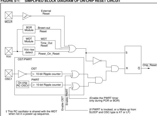
SIMPLIFIED BLOCK DIAGRAM OF ON-CHIP RESET CIRCUIT FIGURE 5-1:
