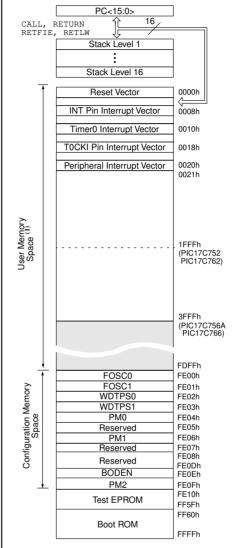
Note 1: User memory space may be internal, external, or both. The memory configuration depends on the processor mode.
