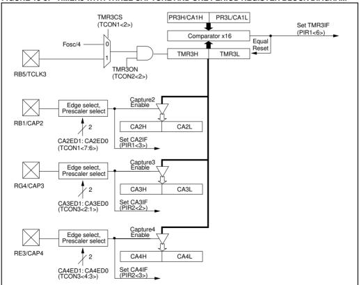
This mode (3 Capture, 1 Period) is selected if control bit CA1/PR3 is clear. In this mode, the Capture1 register, consisting of high byte (PR3H/CA1H) and low byte (PR3L/CA1L), is configured as the period control register for TMR3. Capture1 is disabled in this mode, and the corresponding Interrupt bit CA1IF is never set. TMR3 increments until it equals the value in the period register and then resets to 0000h on the next timer clock.
