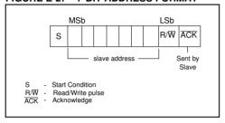
FIGURE E-3: I<sup>2</sup>C 10-BIT ADDRESS FORMAT
