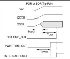
This figure shows in greater detail the timings involved with the oscillator start-up timer. In this example the low frequency crystal start-up time is larger than power-up time (TPWRT).
