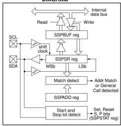
FIGURE 15-3: I<sup>2</sup>C MASTER MODE BLOCK DIAGRAM
