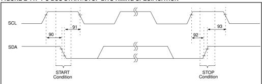
TABLE E-2: I<sup>2</sup>C BUS START/STOP BITS TIMING SPECIFICATION
