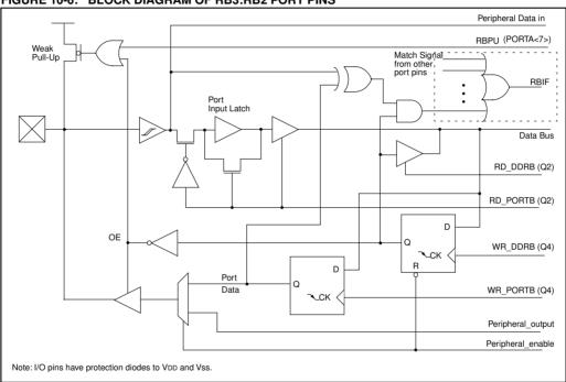
FIGURE 10-7: BLOCK DIAGRAM OF RB6 PORT PIN
