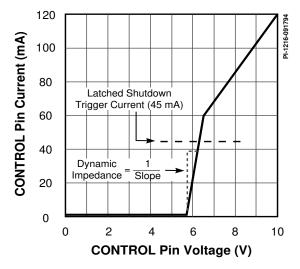
Figure 10. TOPSwitch CONTROL Pin I-V Characteristic.
