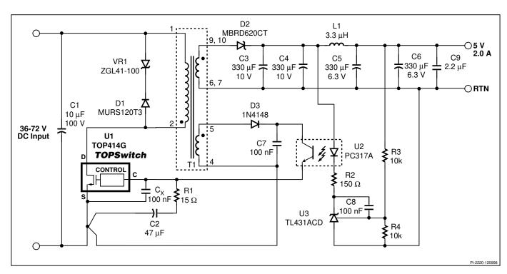
Figure 7. Schematic Diagram of a 5 V, 10 W Isolated DC to DC Converter.
