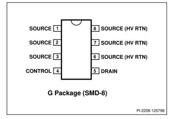
Figure 3. Pin Configuration.
