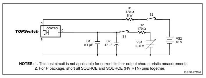
Figure 11. TOPSwitch General Test Circuit.
