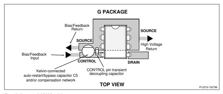
Figure 8. Recommended TOPSwitch Layout.
