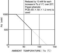
Fig.4 Power dissipation curve (BA6246N, BA6247N)
