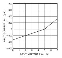
Fig.6 Input voltage vs. input current (BA6246N)
