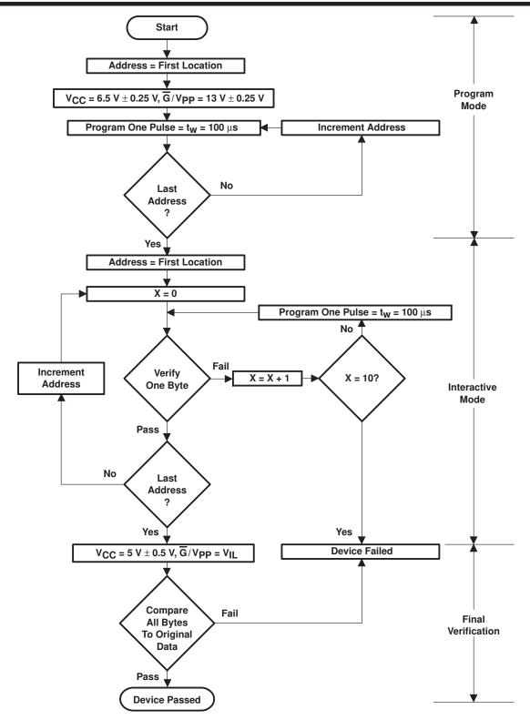
Figure 1. SNAP! Pulse Programming Flow Chart
