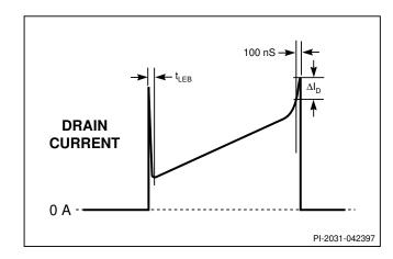
Figure 13. Example of  $\Delta I_{\scriptscriptstyle D}$  on Drain Current Waveform with Saturated Transformer.
