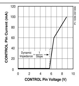
Figure 11. TOPSwitch CONTROL Pin I-V Characteristic.
