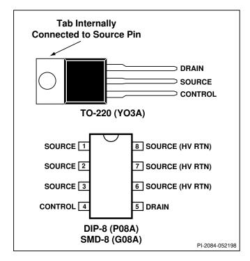
Figure 3. Pin Configuration.
