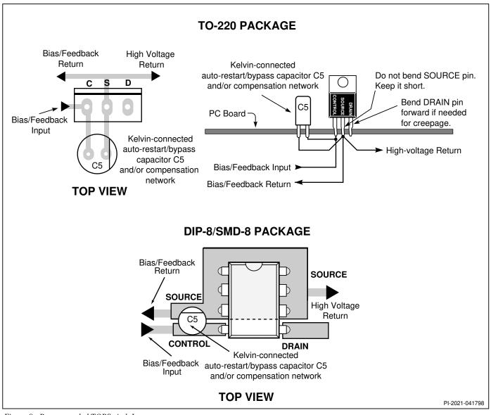
Figure 9. Recommended TOPSwitch Layout.
