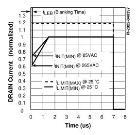
Figure 12. Self-protection Current Limit Envelope.
