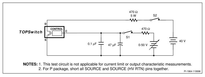
Figure 14. TOPSwitch General Test Circuit.
