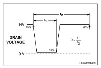
Figure 10. TOPSwitch Duty Cycle Measurement.
