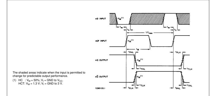
Fig.6 Waveforms showing the clock (nCP) to output (nQ,  $n\overline{Q}$ ) propagation delays, the clock pulse width, the nD to nCP set-up, the nCP to nD hold times, the output transition times and the maximum clock pulse frequency.
