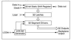
FIGURE 3: BACKPLANE AND SEGMENT OUTPUT
