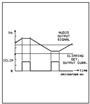
A current sinking at pin 10 is triggered when a certain distortion level is reached at any of the outputs. This function allows gain compression possibility whenever the amplifier is overdriven.
