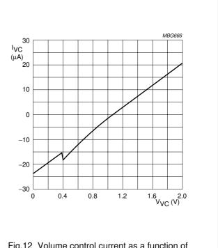
Fig.12 Volume control current as a function of volume control voltage.
