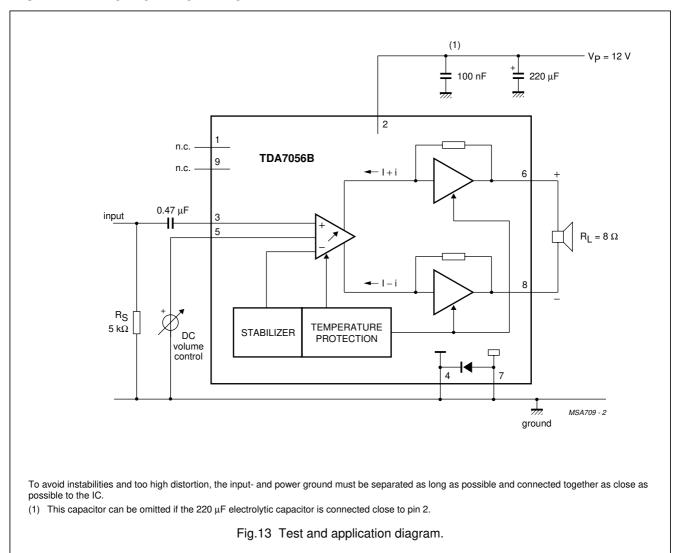
For single-end application the output peak current may not exceed 100 mA; at higher output currents the short circuit protection (MLC) will be activated.
