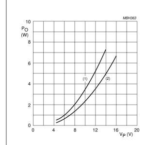
Measured at a THD of 10%. The maximum output power is limited by the maximum power dissipation and the maximum available output current.
