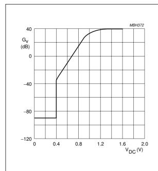
Fig.3 Gain control as a function of DC volume control.
