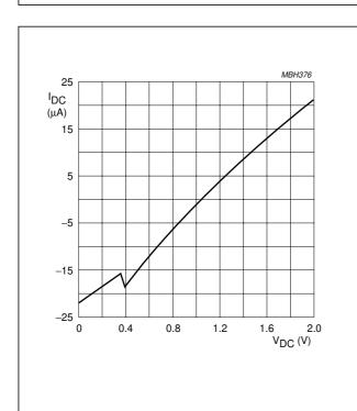
Fig.5 Control current as a function of DC volume control.
