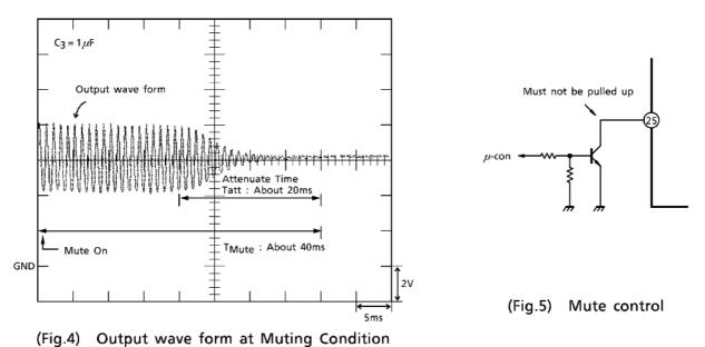
The attenuation by the muting function is 70dB (typ.). This muting is very smooth attenuating by the time constant of pin(1): smoothing.
