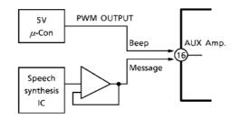
(Fig.7) The application of AUX. amplifier
