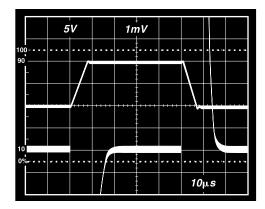
Figure 25. Large Signal Response and Settling Time, G = 100 (0.5 mV = 0.01%)
