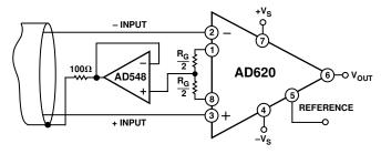
Figure 40. Common-Mode Shield Driver
