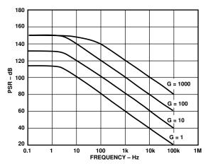
Figure 15. Negative PSR vs. Frequency, RTI (G = 1-1000)
