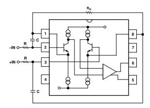
Figure 38. Circuit to Attenuate RF Interference
