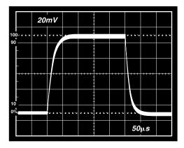
Figure 28. Small Signal Pulse Response, G=1000,  $R_L=2~k\Omega$ ,  $C_L=100~pF$
