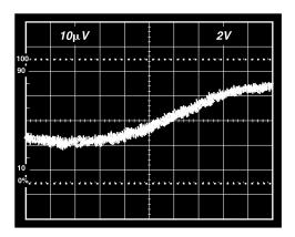
Figure 31a. Gain Nonlinearity, G = 1,  $R_L = 10 \text{ k}\Omega$  (10  $\mu$ V = 1 ppm)
