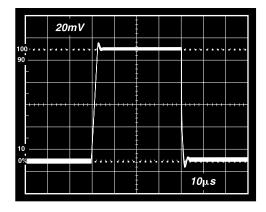
Figure 24. Small Signal Response, G = 10,  $R_L = 2 \text{ k}\Omega$ ,  $C_L = 100 \text{ pF}$
