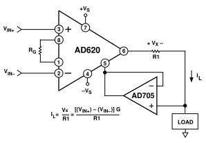
Figure 37. Precision Voltage-to-Current Converter (Operates on 1.8 mA,  $\pm 3$  V)
