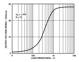
Figure 20. Output Voltage Swing vs. Load Resistance
