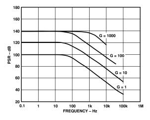
Figure 14. Positive PSR vs. Frequency, RTI (G = 1–1000)
