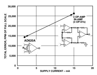
Figure 1. Three Op Amp IA Designs vs. AD620
