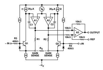
Figure 33. Simplified Schematic of AD620
