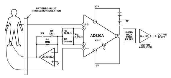
Figure 36. A Medical ECG Monitor Circuit
