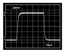
Figure 26. Small Signal Pulse Response, G=100,  $R_L=2~k\Omega$ ,  $C_L=100~pF$
