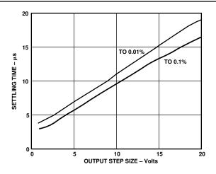
Figure 29. Settling Time vs. Step Size (G = 1)
