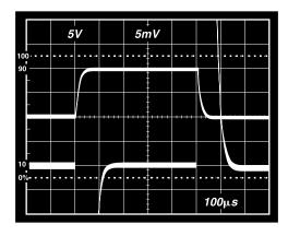
Figure 27. Large Signal Response and Settling Time, G = 1000 (0.5 mV = 0.01%)
