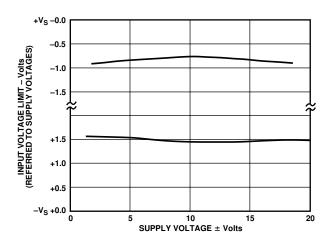
Figure 18. Input Voltage Range vs. Supply Voltage, G = 1
