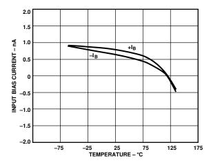
Figure 6. Input Bias Current vs. Temperature
