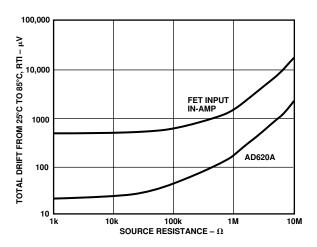
Figure 12. Total Drift vs. Source Resistance
