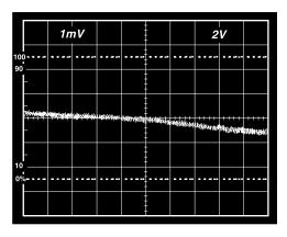
Figure 31c. Gain Nonlinearity,  $G=1000,\,R_L=10~k\Omega$  (1 mV = 100 ppm)
