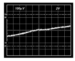
Figure 31b. Gain Nonlinearity, G = 100,  $R_L$  = 10  $k\Omega$  (100  $\mu$  V = 10 ppm)
