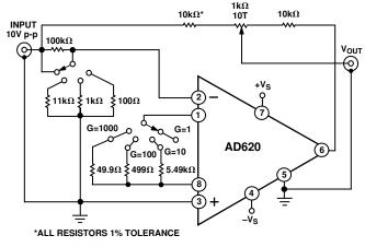
Figure 32. Settling Time Test Circuit
