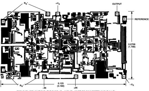
\*FOR CHIP APPLICATIONS: THE PADS  $1R_{\rm G}$  AND  $8R_{\rm G}$  MUST BE CONNECTED IN PARALLEL TO THE EXTERNAL GAIN REGISTER  $R_{\rm G}$ . DO NOT CONNECT THEM IN SERIES TO  $R_{\rm G}$ . FOR UNITY GAIN APPLICATIONS WHERE  $R_{\rm G}$  IS NOT REQUIRED, THE PADS  $1R_{\rm G}$  MAY SIMPLY BE BONDED TOGETHER, AS WELL AS THE PADS  $8R_{\rm G}$ .
