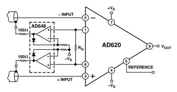
Figure 39. Differential Shield Driver
