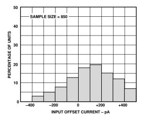
Figure 5. Typical Distribution of Input Offset Current
