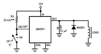
\*\*\* To assure shutdown, select Resistor R3 to ensure at least 300µA of pull-up current when S1 is open. (Assume 2V at the ON/OFF pin.)
