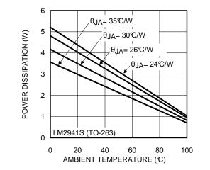
Figure 21. P<sub>D(MAX)</sub> vs T<sub>A</sub> for LM2941S (TO-263)
