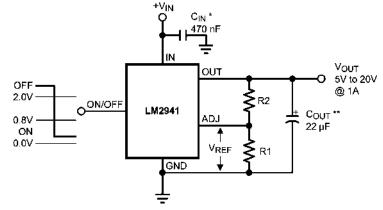
$V_{OUT}$  = Reference voltage  $\sim \frac{R1 + R2}{R1}$  where  $V_{REF} = 1.275$  typical
