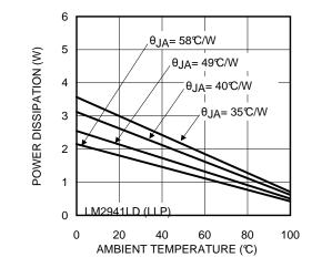
Figure 22. PD<sub>(MAX)</sub> vs T<sub>A</sub> for LM2941LD (WSON)
