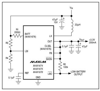
Figure 5. Preset Output Voltage of +3.3V
