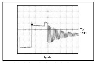
Figure 3. LX Ringing Without Damping Switch
