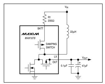
Figure 2. Simplified Diagram of Inductor Damping Switch
