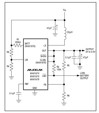
Figure 7. Setting an Adjustable Output
