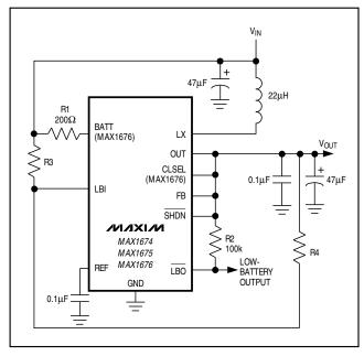
Figure 8. Setting Resistor Values for the Low-Battery Indicator when  $V_{\text{IN}} < 1.3 \text{V}$
