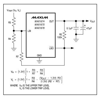
Figure 9. Adding External Hysteresis to the Low-Battery Indicator
