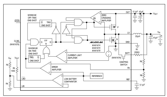
Figure 1. Simplified Functional Diagram
