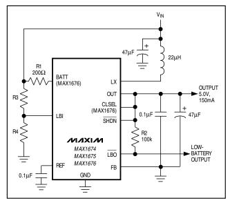
Figure 6. Preset Output Voltage of +5V
