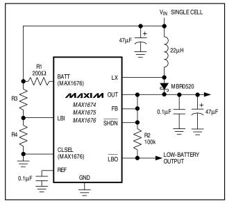
Figure 10. Adding a Schottky Diode for Single-Cell Operation
