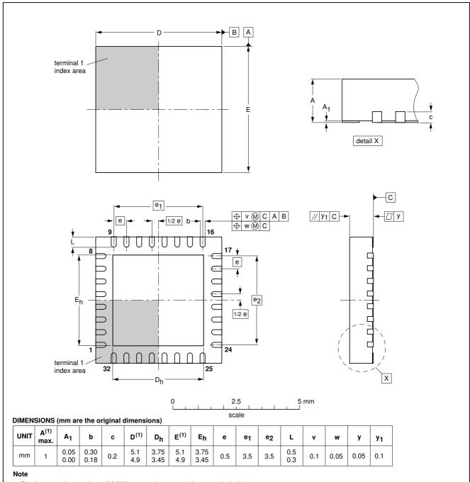
1. Plastic or metal protrusions of 0.075 mm maximum per side are not included.
