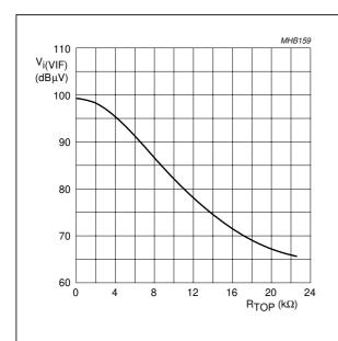
Fig.8 Typical tuner takeover point as a function of resistor  $R_{\text{TOP}}$ .
