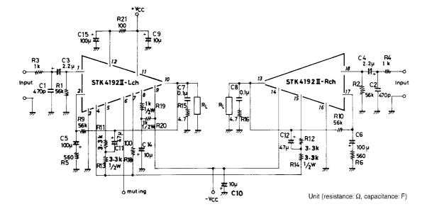
Sample Application Circuit : 50W min 2-channel AF power amplifier
