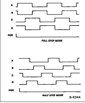
Figure 3 : Input Signal for Stepper Motor Drive.
