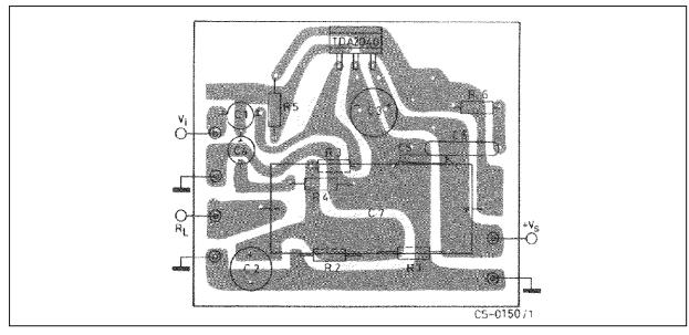
Figure 14: 30W Bridge Amplifier with Split Power Supply
