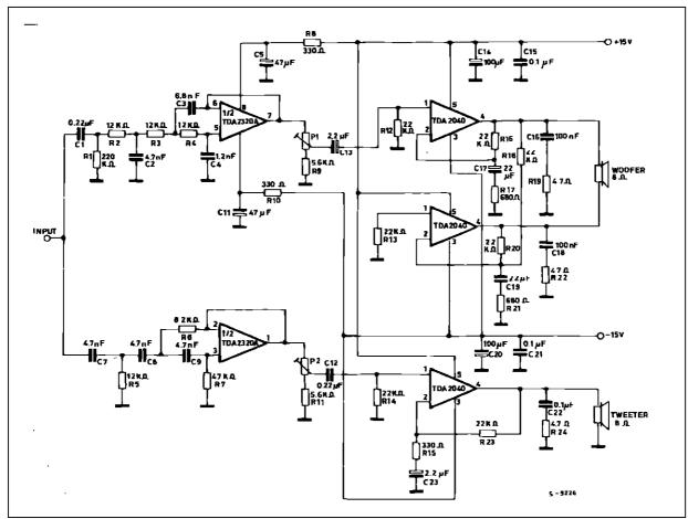
Figure 16: Two Way Hi-Fi System with Active Crossover
