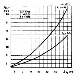
Figure 3: Output Power versus Supply Voltage
