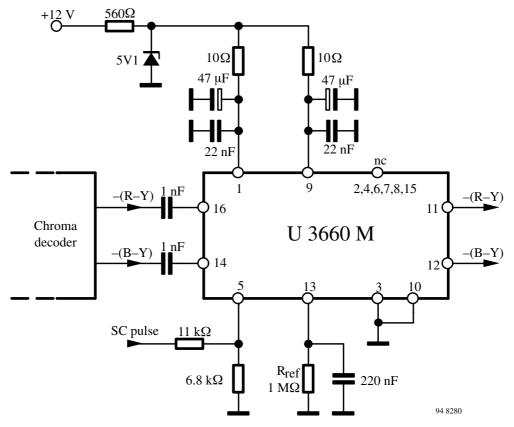
Figure 3. Typical application circuit
