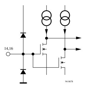
Figure 4. Colour difference signal inputs
