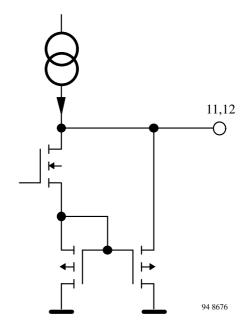
Figure 5. Colour difference signal outputs
