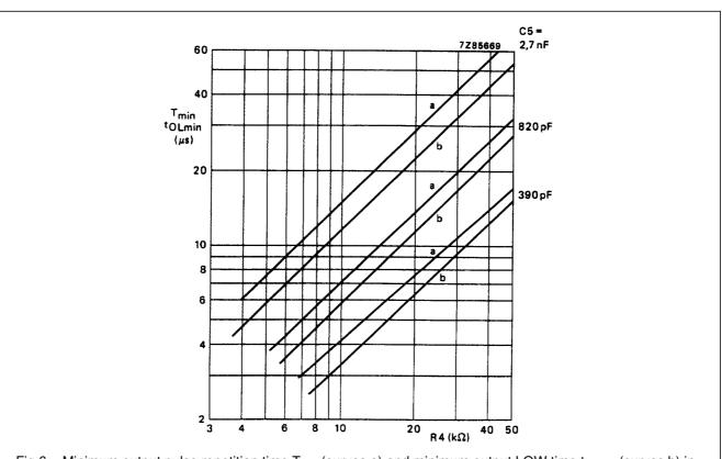
Fig.6 Minimum output pulse repetition time T<sub>min</sub> (curves a) and minimum output LOW time t<sub>OLmin</sub> (curves b) in the frequency regulation mode as a function of external resistor R4 connected between RX and ground with external capacitor C5 connected between CX and ground as a parameter.
