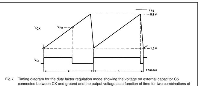
Fig./ Timing diagram for the duty factor regulation mode showing the voltage on external capacitor C5 connected between CX and ground and the output voltage as a function of time for two combinations of input signals. *a:* The voltages on inputs FB or LIM are below 5,9 V. The circuit is in its normal regulation range. *b:* The voltages on inputs FB and LIM are higher than 5,9 V. The circuit produces its minimum output LOW time, giving the maximum duty factor of the SMPS.
