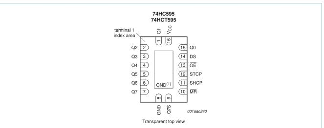
(1) This is not a supply pin, the substrate is attached to this pad using conductive die attach material. There is no electrical or mechanical requirement to solder this pad however if it is soldered the solder land should remain floating or be connected to GND.
