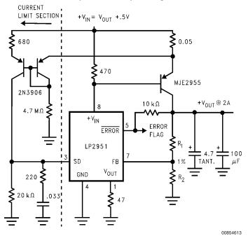
$$V_{out} = 1.23V \left(1 + \frac{R_1}{R_2}\right)$$
