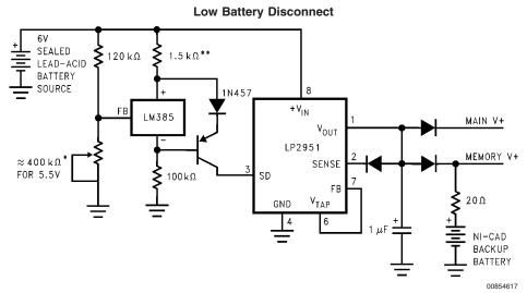
For values shown, Regulator shuts down when  $V_{in}$  < 5.5V and turns on again at 6.0V. Current drain in disconnected mode is  $\approx 150 \mu A$ .
