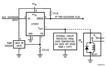
LM34 for 125°F Shutdown LM35 for 125°C Shutdown
