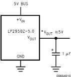
\*Minimum input-output voltage ranges from 40mV to 400mV, depending on load current. Current limit is typically 160mA.
