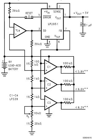
\*Optional Latch off when drop out occurs. Adjust R3 for C2 Switching when  $V_{in}$  is 6.0V.
