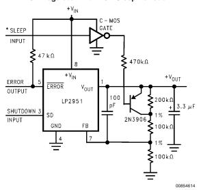
\*High input lowers  $V_{out}$  to 2.5V
