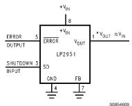
\*Minimum input-output voltage ranges from 40mV to 400mV, depending on load current. Current limit is typically 160mA.
