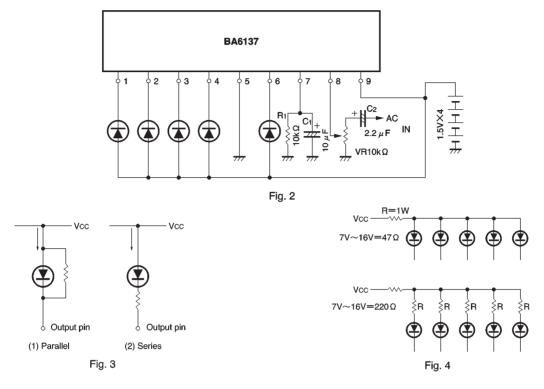
The response time (attack and release time) can be changed by varying the values of  $C_1$  and  $R_1$  to change the time constant.
