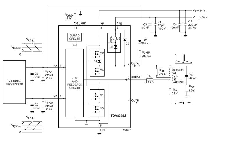
$f_{vert} = 50 \text{ Hz}$ ;  $t_{FB} = 640 \mu s$ ;  $I_{I(bias)} = 400 \mu A$ ;  $I_{i(p-p)} = 290 \mu A$ ;  $I_{o(p-p)} = 2.4 A$ .
