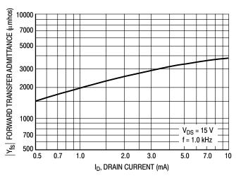
Figure 6.  $V_{GS(off)} = 5.0 \text{ V}$
