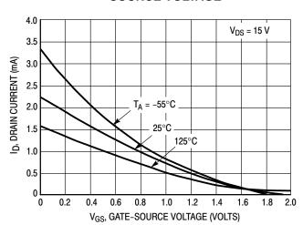
Figure 1. V<sub>GS(off)</sub> = 2.0 V
