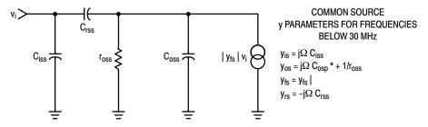
$^*C_{osp}$  is  $C_{oss}$  in parallel with Series Combination of  $C_{iss}$  and  $C_{rss}$ .
