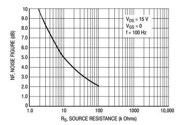
Figure 9. Noise Figure versus Source Resistance
