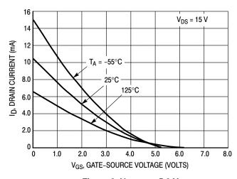
Figure 3.  $V_{GS(off)} = 5.0 \text{ V}$
