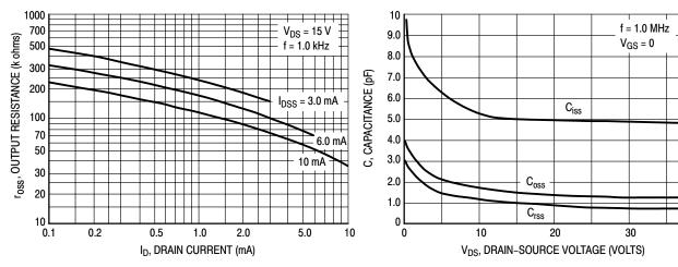
Figure 7. Output Resistance versus Drain Current
