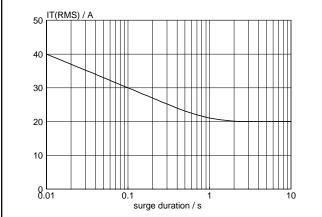
Fig.5. Maximum permissible repetitive rms on-state current  $I_{T(RMS)}$ , versus surge duration, for sinusoidal currents, f = 50 Hz;  $T_{hs} \le 43$  °C.
