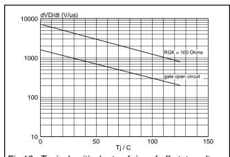
Fig.12. Typical, critical rate of rise of off-state voltage, dV<sub>D</sub>/dt versus junction temperature T<sub>j</sub>.
