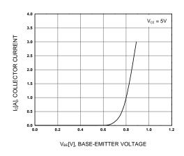
Figure 4. Base-Emitter On Voltage
