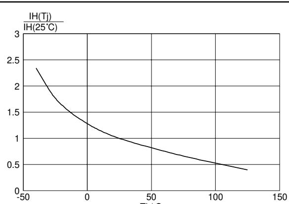
Fig.9. Normalised holding current  $I_H(T_j)/I_H(25^\circ C)$ , versus junction temperature  $T_j$ .
