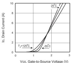
Figure 2. Transfer Characteristics
