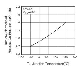
Figure 4. On-Resistance Variation with Temperature
