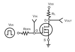
Figure 9. Switching Test Circuit
