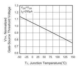
Figure 5. Gate Threshold Variation with Temperature
