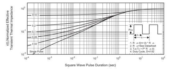
Figure 11. Normalized Thermal Transient Impedance Curve
