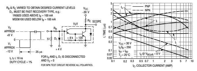
Figure 9. Switching Times Test Circuit
