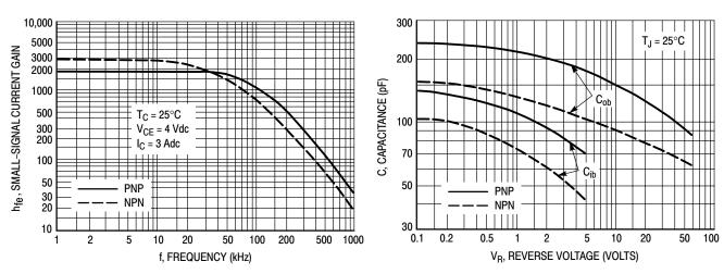
Figure 7. Small-Signal Current Gain
