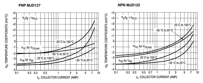
**Figure 5. Temperature Coefficients**
