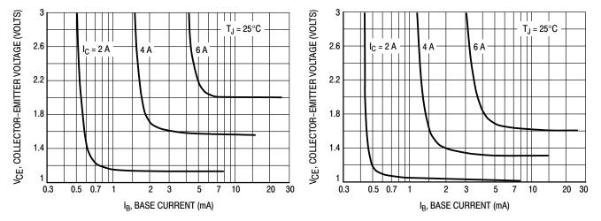
Figure 3. Collector Saturation Region
