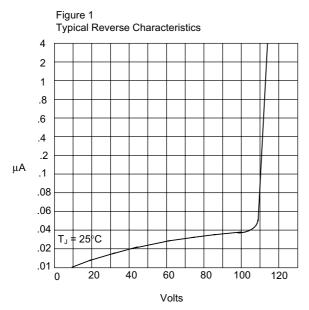
Instantaneous Reverse Current - Micro Ampsversus Percent Of Rated Peak Reverse Voltage - Volts
