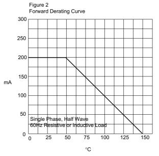
Average Forward Rectified Current - Amperes/ersus Ambient Temperature -°C
