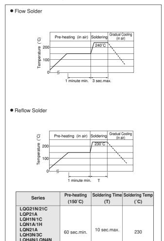
(5) Reworking with Soldering Iron Preheating at 150°C for 1 minute is required. Do not directly touch the ceramic element with the tip of the soldering iron. The reworking soldering conditions are as follows.
