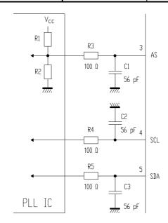
Fig.4 I<sup>2</sup>C-bus load.
