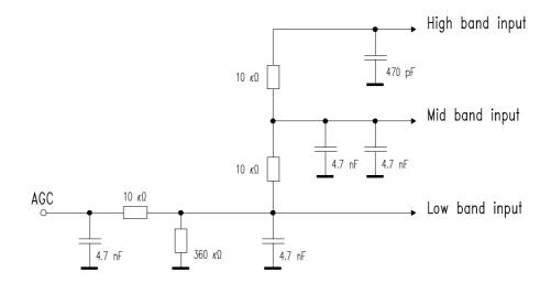
Fig.5 Internal AGC circuit.
