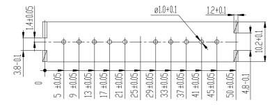
Fig.8 Punching pattern seen from solder side
